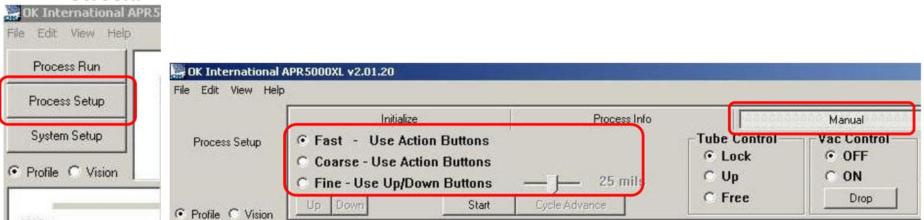
The Fast/Coarse/Fine are speeds for moving the z-axis head up and down using the UP – DOWN buttons on front of the machine. Both buttons for either UP or DOWN must be depressed at same time in order to move the head.
